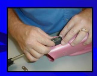
Place stainless top cover onto mount and insert two stainless screws and tighten, always check screws prior to diving
